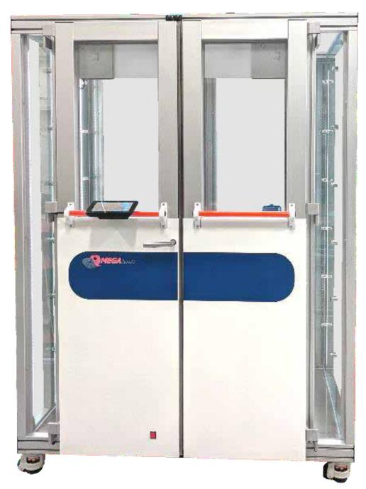
Fingerprint fuming chamber for Cyanoacrylate development of fingers on non-porous surfaces
